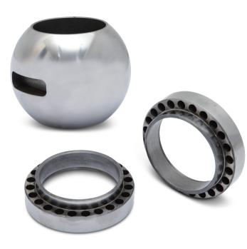
Scraper seat design Protects sealing surface of ball seat Removes particles, foreign object, slurry, etc. High Hardness of over HV2,000 Pocketless Design Prevents buildup of solids inside the valve's body dead space
